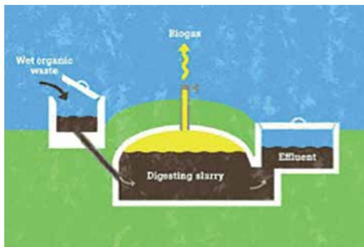
Figure 2: Basic components of a fixed-dome biogas digester plant
